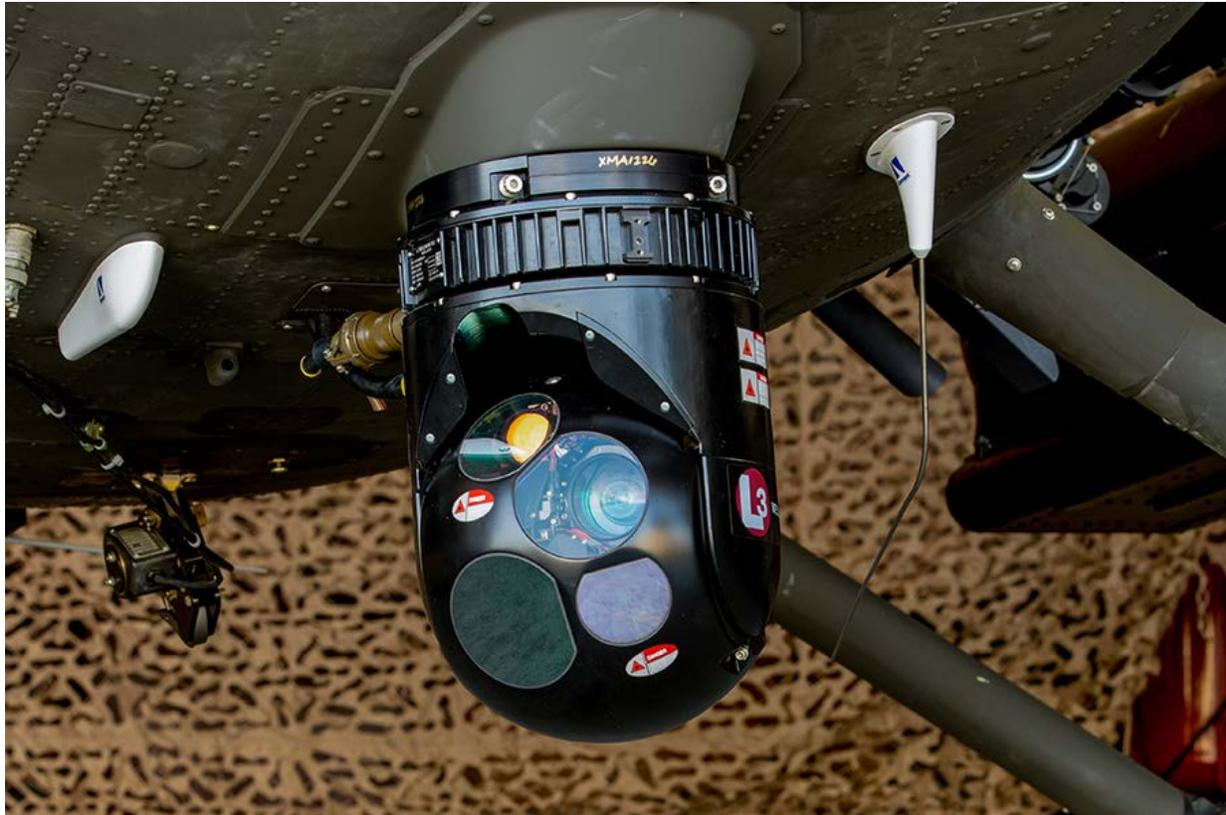
The [L-3](#) Wescam MX-10 series sensor and LASER designator will round out the MD 530G mission and weapons equipment package.
