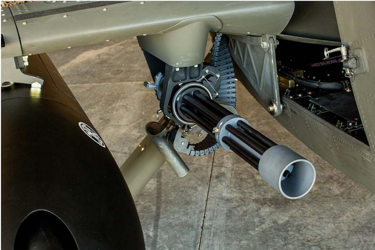
The MD 530G's light machine gun solution is the [Dillon Aero](#) M134D-H Gatling Gun.
